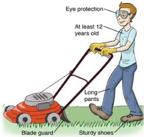
Appropriate clothing should be worn. This includes sturdy, closed-toe shoes, safety glasses, and hearing protection.
